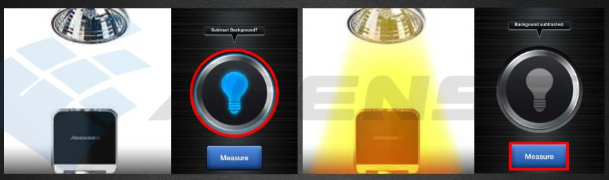
Step 1 : Turn off the light source before measuring.Step 2 : Press "Subtract Background" button. (The button will then grays out.)Step 3 : Turn on the light source for a while, then press the "Measure" button.
